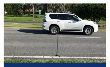
The majority of all count stations in Marion County are temporary count stations. These sites feature a portable count computer and pneumatic tubes that are taped across the roadway. When driven over, a burst of air pressure is sent through the tube to the counter. For each vehicle that passes over the tubes, the counter records the time of occurance. Permanent Stations
